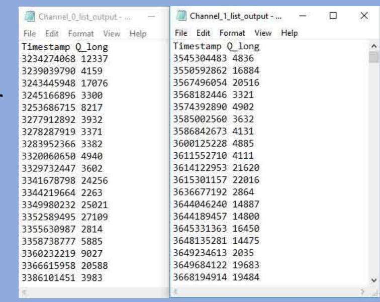
CAEN. Thus, whenever the FPGAs trigger an output event, information about the triggered event is then written to a specified PC .txt file. This is shown in the example for two gamma ray detectors with coincident events.
