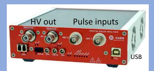
though configuration files which write logic to the channels registers in order to perform acquisition that involves pulse discrimination or coincidence timing.
