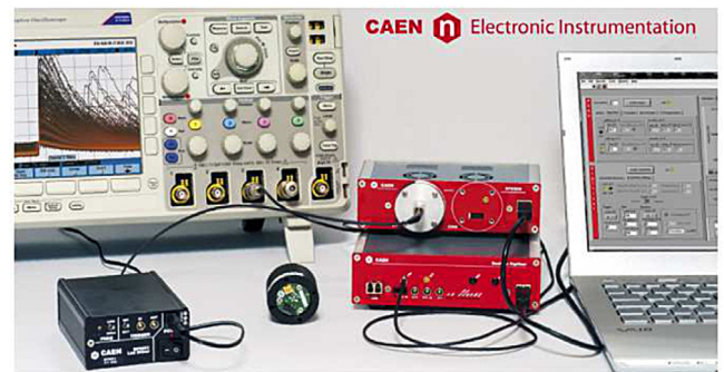
Fig. 8. CAEN setup (Ref. [24]) for the characterisation of SiPMs. It is a modular plug-and-play system which is simple to set up and allows characterising many properties of SiPMs. A suite of analysis software comes with the system. Similar systems are also available from other vendors. These systems are ideal for a first step towards characterising SiPMs and also well suited for laboratories for pupils and students.
