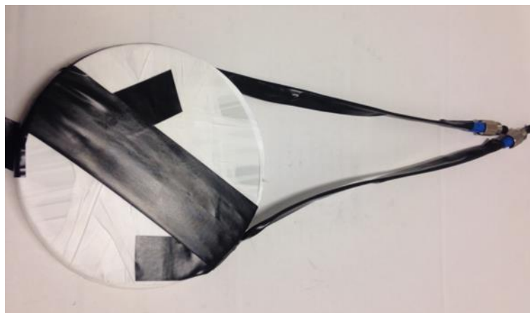
Figure 5. White thread sealing tape and black electrical tape surrounding the plastic scintillator disc NE102A.
