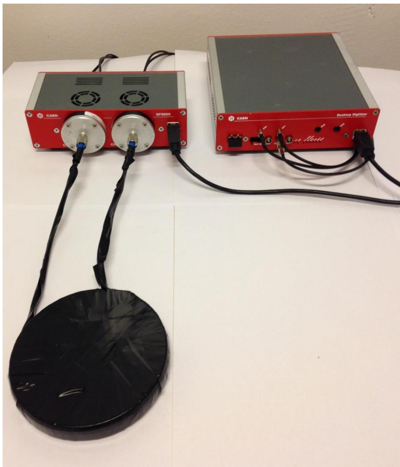
Figure 7. Light protected plastic scintillator NE102A with WLS-fibre BCF-92 connected with FC-connectors to SP5600 General Purpose Power Supply and Amplification Unit. The signal from SP5600 is processed in DT5720A Desktop Digitizer and two USB-cables are connected to a PC.
