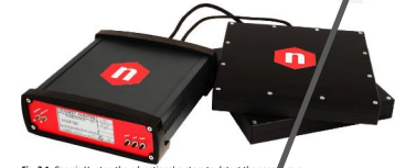
Fig. 2.1: Cosmic Hunter, the educational system to detect the cosmic rays.
