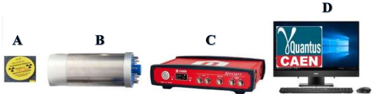
Figure 0: Scheme of the experimental setup: radioactive source (A) in front of the inorganic scintillator (B), which is connector to the MCA Hexagon (C) ( see more here ) supplied by the software Quantus (D).
