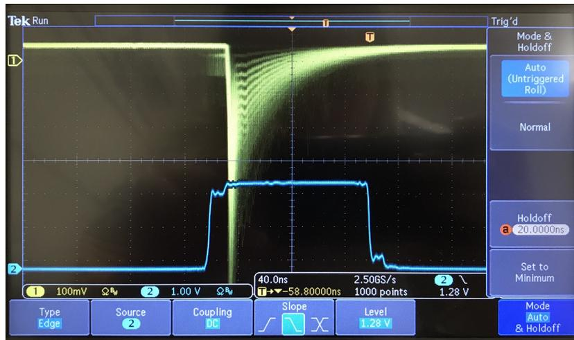
Figure 21: A multi-photon peak spectrum with triggering on the LED driver output signal on channel 2. Channel 1 is set to 100 mV scale, channel 2 is set to 1 V scale and the horizontal scale is 40 ns. Trigger threshold is set to 1.28V on channel 2 in the example here.
