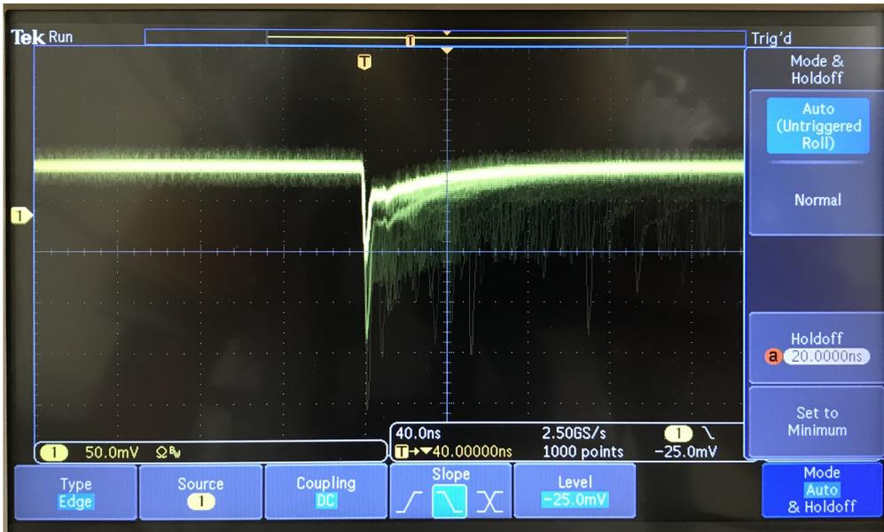
Figure 20: Example of the SiPM output signal at a gain of 40 dB for a sensor with no LED light. Horizontal scale is set to 40 ns (trigger menu - horizontal scale and vertical scale is set to 50 mV (use channel menu to set it).
