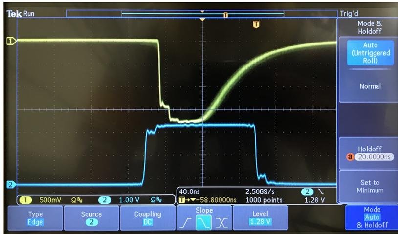
Figure 22: Example of the saturation region of the SiPM. Channel 1 is set to 500 mV scale, channel 2 is set to 1 V scale and the horizontal scale is 40 ns. Trigger threshold is set to 1.28V on channel 2 in the example here.
