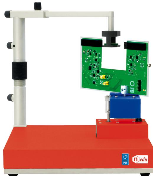
Fig. 2. The easyPET educational prototype constituted by two stepper motors, a U-shaped PCB equipped with two detecting units and a source holder.
