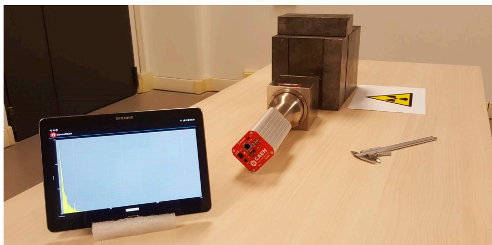
Figure 3. Experimental setup for the indoor experiment: on the left the tablet showing the graphical interface of the GammaTOUCH app during the acquisition, on the right the 4" \times 4" NaI(Tl) detector and the lead box.
