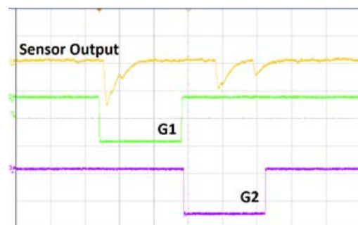
Fig. 1: The figure shows the response of the SiPM to a light burst, synchronised with the leading edge of the gate G_1 . Pulses in the G_2 gate may be due to both random Dark Counts and after-pulses. The exemplary event shown here features as well an after-pulse occurring during the recovery time of the sensor. The rate of Dark Counts is measured switching off the LED.
