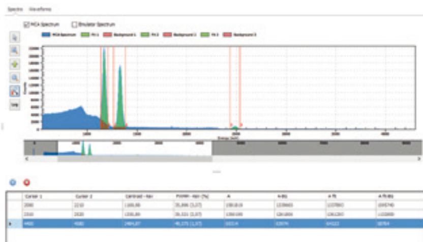
The ^{60}\text{Co} complete spectrum acquired by the MCA DT5770 and plotted by the Emulation Software
