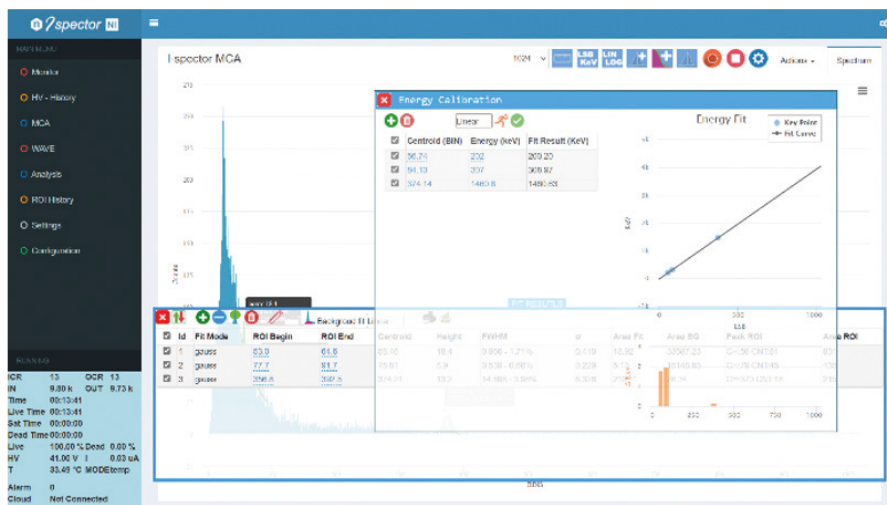
Linear dependency in the Energy Calibration.
